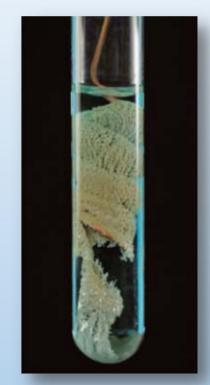
$2A1+3CuSO_4===A1_2(SO_4)_3+3Cu$  |  $Cu+2AgNO_3===Cu(NO_3)_2+2Ag$
